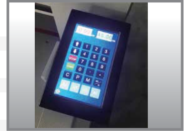
▲ 99 programs with 10 steps each repeat cut function and push out function, touch screen
